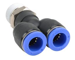
NITRA pneumatic push-to-connect fitting, Y, rotating, thermoplastic (PBT) body, nickel-plated brass threads, thread sealant, (1) R1/2 male BSPT to (2) 12mm push-to-connect. Package of 5.
