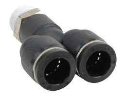
NITRA pneumatic push-to-connect fitting, Y, rotating, thermoplastic (PBT) body, nickel-plated brass threads, thread sealant, (1) 3/8in male NPT to (2) 1/2in push-to-connect. Package of 5.
