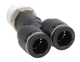
NITRA pneumatic push-to-connect fitting, Y, rotating, thermoplastic (PBT) body, nickel-plated brass threads, thread sealant, (1) 1/4in male NPT to (2) 1/2in push-to-connect. Package of 5.
