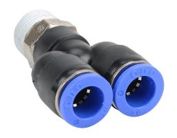
NITRA pneumatic push-to-connect fitting, Y, rotating, thermoplastic (PBT) body, nickel-plated brass threads, thread sealant, (1) R3/8 male BSPT to (2) 10mm push-to-connect. Package of 5.
