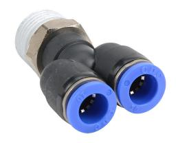
NITRA pneumatic push-to-connect fitting, Y, rotating, thermoplastic (PBT) body, nickel-plated brass threads, thread sealant, (1) R1/2 male BSPT to (2) 10mm push-to-connect. Package of 5.
