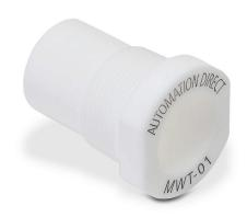
AutomationDirect sensor mounting well, PTFE body, 1-1/4in male NPT process connection, 30mm bore, 2.55in overall length, 2.07in insertion length.
