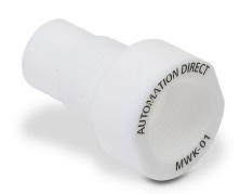
AutomationDirect sensor mounting well, PTFE body, 3/4in male NPT process connection, 18mm bore, 2.25in overall length, 1.50in insertion length.
