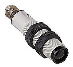
AutomationDirect photoelectric sensor, tubular, threaded, polarized retroreflective, visible red light emission, 3m sensing distance, dark-on, 3-wire, 4-pin M12 quick-disconnect.
