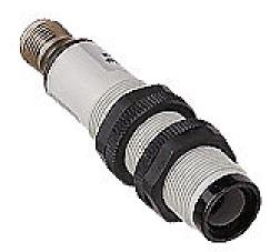
AutomationDirect photoelectric sensor, tubular, threaded, plastic housing, through-beam emitter, infrared light emission, 16m sensing distance, 20-253 VAC operating voltage, 2-wire, 4-pin M12 quick-disconnect.
