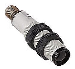
AutomationDirect photoelectric sensor, tubular, threaded, diffuse, infrared light emission, 400mm sensing distance, light-on, 25 Hz switching frequency, plastic housing, 4-pin M12 quick-disconnect.
