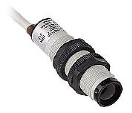
AutomationDirect photoelectric sensor, tubular, threaded, diffuse, infrared light emission, 400mm sensing distance, light-on, 25 Hz switching frequency, plastic housing, pigtail.
