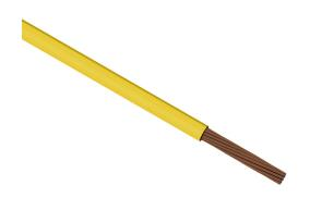
Direct Wire All-Flex flexible power cable, unshielded, MTW and THHW, single conductor, 8 AWG, bare copper, PVC conductor insulation material, yellow, cut to length.
