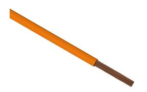
Direct Wire All-Flex flexible power cable, unshielded, MTW and THHW, single conductor, 8 AWG, bare copper, PVC conductor insulation material, orange, cut to length.
