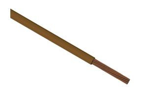
Direct Wire All-Flex flexible power cable, unshielded, MTW and THHW, single conductor, 8 AWG, bare copper, PVC conductor insulation material, brown, cut to length.
