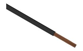
Direct Wire flexible power cable, unshielded, MTW and THHW, single conductor, 8 AWG, bare copper, PVC conductor insulation material, black, cut to length.
