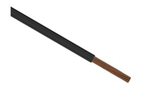
Direct Wire flexible power cable, unshielded, MTW and THHW, single conductor, 8 AWG, bare copper, PVC conductor insulation material, black, cut to length.
