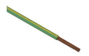
Direct Wire All-Flex flexible power cable, unshielded, MTW and THHW, single conductor, 6 AWG, bare copper, PVC conductor insulation material, green with yellow stripe, cut to length.
