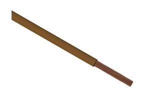
Direct Wire All-Flex flexible power cable, unshielded, MTW and THHW, single conductor, 6 AWG, bare copper, PVC conductor insulation material, brown, cut to length.
