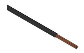
Direct Wire flexible power cable, unshielded, MTW and THHW, single conductor, 6 AWG, bare copper, PVC conductor insulation material, black, cut to length.
