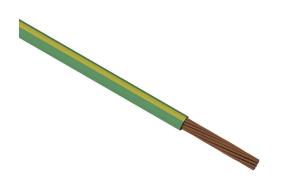
Direct Wire All-Flex flexible power cable, unshielded, MTW and THHW, single conductor, 4 AWG, bare copper, PVC conductor insulation material, green with yellow stripe, cut to length.
