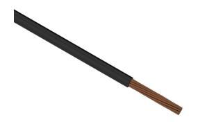
Direct Wire flexible power cable, unshielded, MTW and THHW, single conductor, 4 AWG, bare copper, PVC conductor insulation material, black, cut to length.
