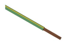
Direct Wire All-Flex flexible power cable, unshielded, MTW and THHW, single conductor, 4/0 AWG, bare copper, PVC conductor insulation material, green with yellow stripe, cut to length.
