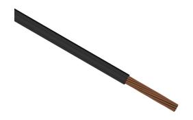
Direct Wire flexible power cable, unshielded, MTW and THHW, single conductor, 4/0 AWG, bare copper, PVC conductor insulation material, black, cut to length.
