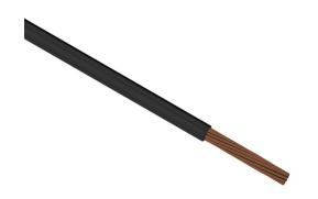
Direct Wire flexible power cable, unshielded, MTW and THHW, single conductor, 2 AWG, bare copper, PVC conductor insulation material, black, cut to length.
