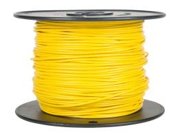
Atlas Wire MTW hook-up wire, single conductor, 22 AWG, 7-stranded, bare copper, PVC conductor insulation material, yellow, 600V, 500ft spool.
