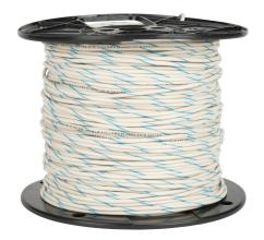
Atlas Wire MTW hook-up wire, single conductor, 22 AWG, 7-stranded, bare copper, PVC conductor insulation material, white with blue stripe, 600V, 500ft spool.
