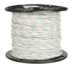
Atlas Wire MTW hook-up wire, single conductor, 22 AWG, 7-stranded, bare copper, PVC conductor insulation material, white with blue stripe, 600V, 1000ft spool.
