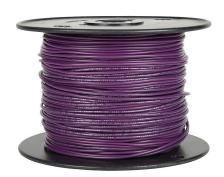
Atlas Wire MTW hook-up wire, single conductor, 22 AWG, 7-stranded, bare copper, PVC conductor insulation material, purple, 600V, 500ft spool.
