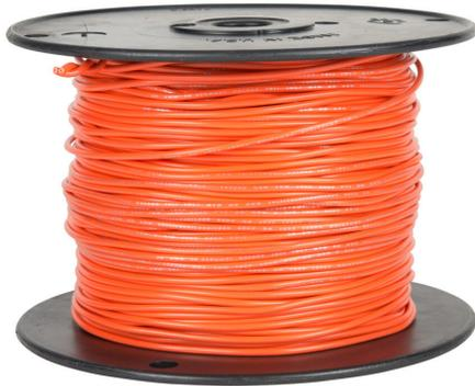
Atlas Wire MTW hook-up wire, single conductor, 22 AWG, 7-stranded, bare copper, PVC conductor insulation material, orange, 600V, 500ft spool.
