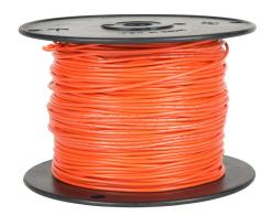
Atlas Wire MTW hook-up wire, single conductor, 22 AWG, 7-stranded, bare copper, PVC conductor insulation material, orange, 600V, 1000ft spool.
