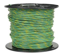
Atlas Wire MTW hook-up wire, single conductor, 22 AWG, 7-stranded, bare copper, PVC conductor insulation material, green with yellow stripe, 600V, 500ft spool.
