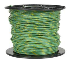
Atlas Wire MTW hook-up wire, single conductor, 22 AWG, 7-stranded, bare copper, PVC conductor insulation material, green with yellow stripe, 600V, 500ft spool.
