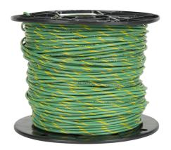
Atlas Wire MTW hook-up wire, single conductor, 22 AWG, 7-stranded, bare copper, PVC conductor insulation material, green with yellow stripe, 600V, 1000ft spool.
