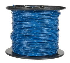
Atlas Wire MTW hook-up wire, single conductor, 22 AWG, 7-stranded, bare copper, PVC conductor insulation material, blue with white stripe, 600V, 500ft spool.
