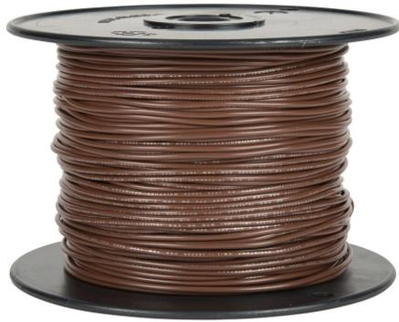
Atlas Wire MTW hook-up wire, single conductor, 22 AWG, 7-stranded, bare copper, PVC conductor insulation material, brown, 600V, 500ft spool.
