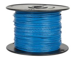
Atlas Wire MTW hook-up wire, single conductor, 22 AWG, 7-stranded, bare copper, PVC conductor insulation material, blue, 600V, 1000ft spool.
