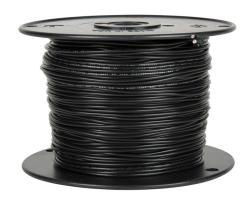
Atlas Wire MTW hook-up wire, single conductor, 22 AWG, 7-stranded, bare copper, PVC conductor insulation material, black, 600V, 1000ft spool.
