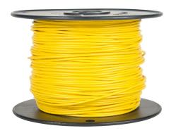
Atlas Wire MTW hook-up wire, single conductor, 20 AWG, 10-stranded, bare copper, PVC conductor insulation material, yellow, 600V, 500ft spool.
