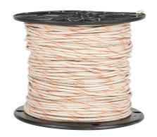
Atlas Wire MTW hook-up wire, single conductor, 20 AWG, 10-stranded, bare copper, PVC conductor insulation material, white with orange stripe, 600V, 500ft spool.
