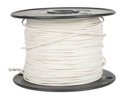
Atlas Wire MTW hook-up wire, single conductor, 20 AWG, 10-stranded, bare copper, PVC conductor insulation material, white, 600V, 1000ft spool.
