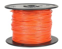
Atlas Wire MTW hook-up wire, single conductor, 20 AWG, 10-stranded, bare copper, PVC conductor insulation material, orange, 600V, 1000ft spool.
