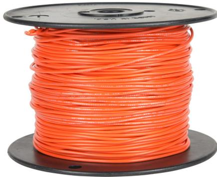
Atlas Wire MTW hook-up wire, single conductor, 20 AWG, 10-stranded, bare copper, PVC conductor insulation material, orange, 600V, 1000ft spool.
