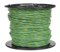
Atlas Wire MTW hook-up wire, single conductor, 20 AWG, 10-stranded, bare copper, PVC conductor insulation material, green with yellow stripe, 600V, 1000ft spool.
