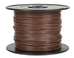
Atlas Wire MTW hook-up wire, single conductor, 20 AWG, 10-stranded, bare copper, PVC conductor insulation material, brown, 600V, 500ft spool.
