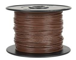
Atlas Wire MTW hook-up wire, single conductor, 20 AWG, 10-stranded, bare copper, PVC conductor insulation material, brown, 600V, 1000ft spool.
