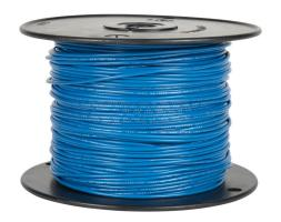
Atlas Wire MTW hook-up wire, single conductor, 20 AWG, 10-stranded, bare copper, PVC conductor insulation material, blue, 600V, 500ft spool.
