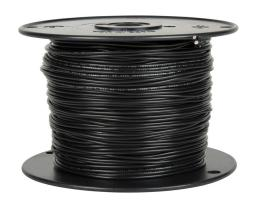
Atlas Wire MTW hook-up wire, single conductor, 20 AWG, 10-stranded, bare copper, PVC conductor insulation material, black, 600V, 1000ft spool.
