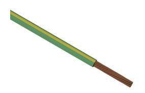
Direct Wire All-Flex flexible power cable, unshielded, MTW and THHW, single conductor, 2/0 AWG, bare copper, PVC conductor insulation material, green with yellow stripe, cut to length.
