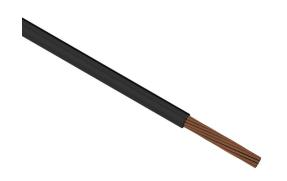
Direct Wire flexible power cable, unshielded, MTW and THHW, single conductor, 2/0 AWG, bare copper, PVC conductor insulation material, black, cut to length.
