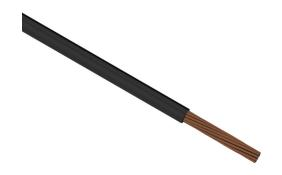
Direct Wire flexible power cable, unshielded, MTW and THHW, single conductor, 1 AWG, bare copper, PVC conductor insulation material, black, cut to length.
