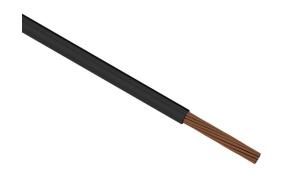
Direct Wire flexible power cable, unshielded, MTW and THHW, single conductor, 1 AWG, bare copper, PVC conductor insulation material, black, cut to length.
