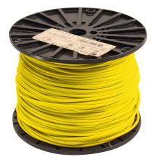
Atlas Wire MTW hook-up wire, single conductor, 18 AWG, 16-stranded, bare copper, PVC conductor insulation material, yellow, 600V, 500ft spool.
