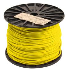
Atlas Wire MTW hook-up wire, single conductor, 18 AWG, 16-stranded, bare copper, PVC conductor insulation material, yellow, 600V, 1000ft spool.
