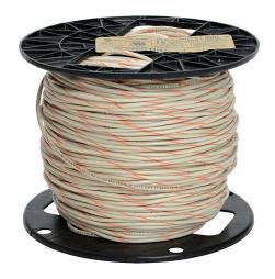
Atlas Wire MTW hook-up wire, single conductor, 18 AWG, 16-stranded, bare copper, PVC conductor insulation material, white with orange stripe, 600V, 500ft spool.
