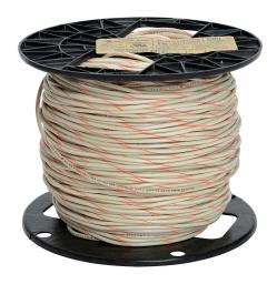
Atlas Wire MTW hook-up wire, single conductor, 18 AWG, 16-stranded, bare copper, PVC conductor insulation material, white with orange stripe, 600V, 500ft spool.
